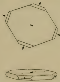
Fig. 17. A Crystal of Barite showing the Symmetry of Orthorhombic Crystals.
